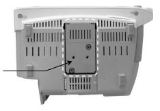
1. Fasten Philips-supplied Table Top Mount to Mounting Adapter with one (1) M6 x 12mm FHMS and two (2) M6 x 8mm FHMS (see below).
