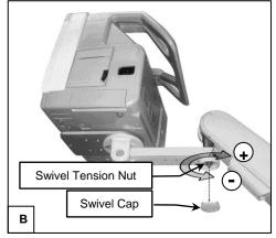
7.4 Rear Pivot Tension Adjustment – To adjust the tension at the rear Pivot Point (closest to channel), tighten (+) or loosen (-) the Pivot Tension Nut with a 3/4" or a 19 mm socket wrench until desired tension is achieved. Do not remove the Pivot Tension Nut.
