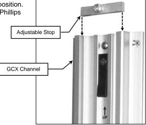
**4.2** While supporting the bottom of the VHM-25 Arm, guide the Slide into the top of the Channel (right) and position it against the Adjustable Stop.
