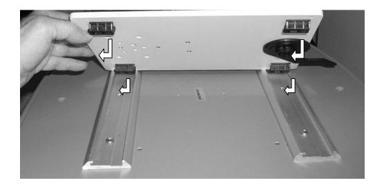
2. Lock Camlock Plate by moving Camlock Lever from right to left. To prevent Camlock Lever from being unlocked, insert one (1) #6-32 x 3/8" PHMS in the threaded hole to the right of the Lever (below right). To further secure the Camlock Mount in the Rails, insert one (1) M4 x 20mm PHMS in each of the two (2) threaded holes at the rear corners of the Mount (below right). Stop tightening these screws when they make contact with the bottom of the Rail.
