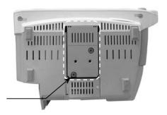
Do Not Attach Table Top Mount if MP20/30 Monitor is Equipped with This Mounting Interface
