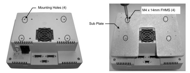
3. Locate four (4) threaded mounting holes on the Subplate (below left). Fasten the Subplate to the display arm with four (4) M4 x 8mm PHMS.
