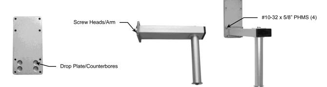
2. Attach Drop Plate to Slide Plate using four (4) #10-32 x 3/4" PHMS (below center and right). Clamp module rack (or other device with clamp) to the Post.
