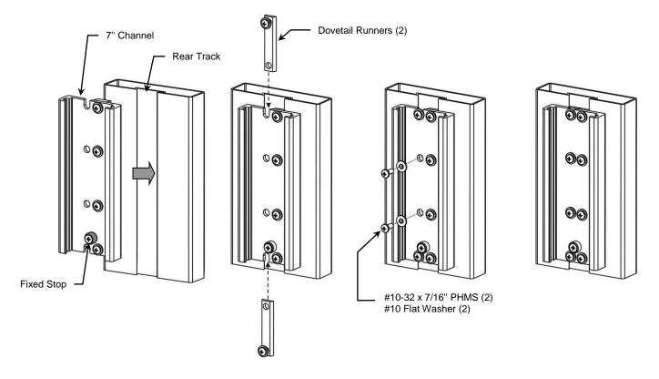
Position the bottom of Channel 1.25" above the base of the machine or existing counterweight (see photo). Tighten all eight (8) screws in the 7" Channel.
