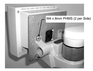
Locate four (4) mounting holes on the Subplate (below left). Fasten Mounting Bracket to Subplate with four (4) M4 x 12mm PHMS. Installation Note: An additional set of mounting holes is provided if additional height is required for the monitor (indicated by triangle in photo below left).
