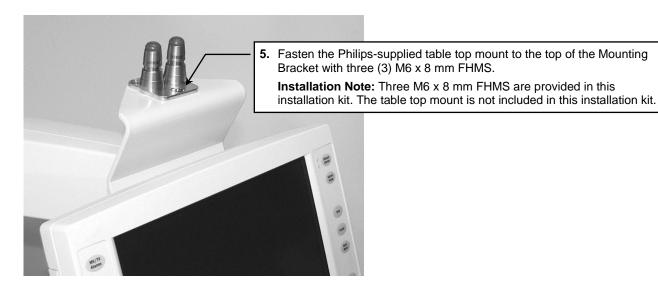
**CAUTION!** Before mounting the Philips MP70 Display on the Mounting Bracket, ensure there is adequate friction being applied to both Wrist Casting Bearing Housings by torquing, uniformly, each clamping screw on the 2 Bearing Housings. The appropriate friction shall be able to prevent the Philips MP70 Display from rotating forward without assistance of the user.
