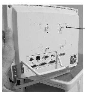
3. Thread four (4) M4 x 12mm SHCS into the mounting holes of the 75mm VESA mounting pattern on rear of ventilator display. Leave 8mm of thread exposed for inserting screw heads through keyholes in Mounting Bracket.
