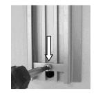
2. While supporting the bottom of the Arm, guide the Slide (at rear of Arm) into the top of the wall channel. Slide the Arm to the desired position in the channel and tighten two (2) set screws (bottom of the Slide) using the 1/8" key. The M-Series Arm should be securely mounted as shown below right.
