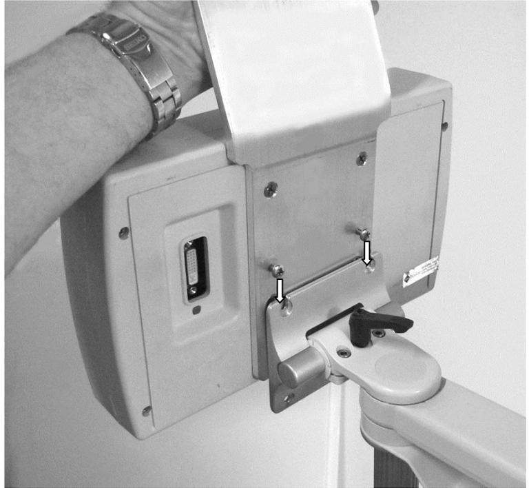
4. Install two (2) #10-32 x 3/8" PHMS into lower mounting holes (shown below) and tighten all four (4) mounting screws.
