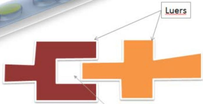
Luers on other cannulas can have too much dead air space, causing turbulence in sample stream. Wave forms are then rounded especially at higher respiratory rates.
