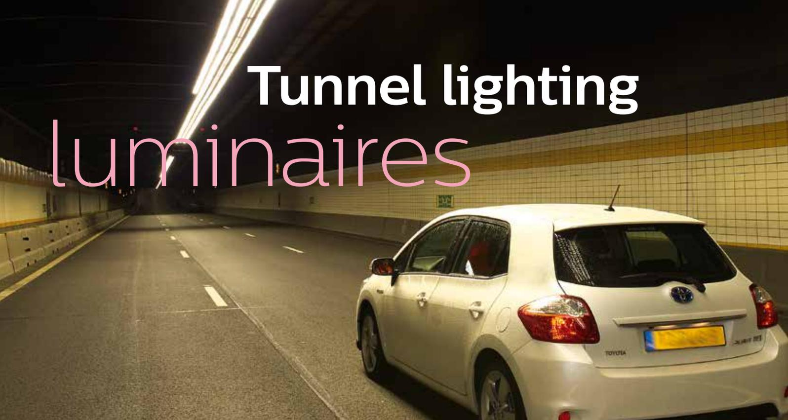
Each zone within a tunnel has its own requirements in terms of lighting design and performance. For example, tunnel entrances require high levels of light with little or no luminaire spacing. In contrast, the lighting in the tunnel interior should be a low level with or without luminaire spacing. With our extensive portfolio of luminaires we can create any lighting concept to provide exactly the right balance between visibility, safety and costs.
