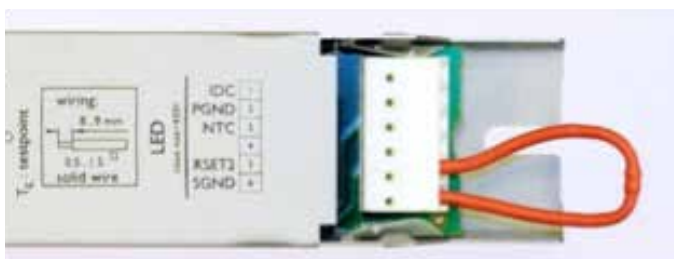
Example of an insulated Rset
