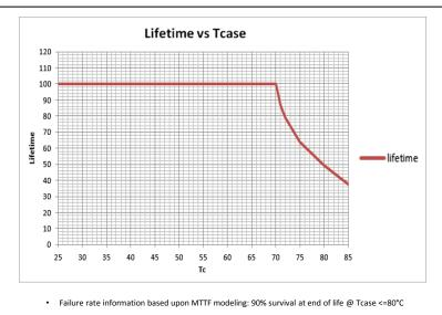
• Failure rate information based upon field call rate data: <0.01% per 1K hour @ Tcase <=80°C
