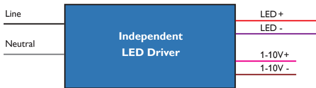
LED driver with 1-10V dimming interface
