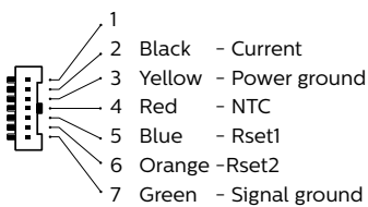
JST connector (driver side) pin layout 75 W & 110 W
