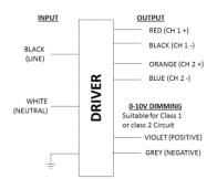
Input lead wires are 18AWG 105C/600V stranded copper with flag terminals per UL1452.
