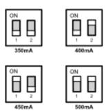
The driver will be shipped out of factory with both switches set to ON (500mA).
