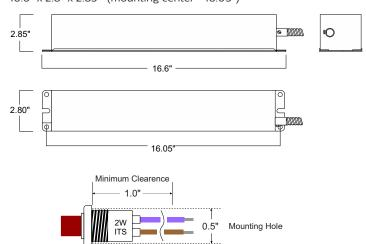
An illuminated test switch/charging indicator light is provided.
