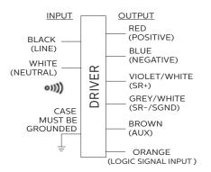
Input and output use lead-wires.
