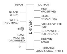
Input and output use lead-wires.
