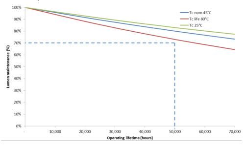
Lumen depreciation as a function of operating hours for I-life and Tc. 50,000 hours proven by certified laboratory.
