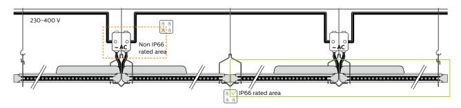
The "none IP rated area", must be build into an >IP66 environment. E.g. into a water tight junction box or water tight connectors.
