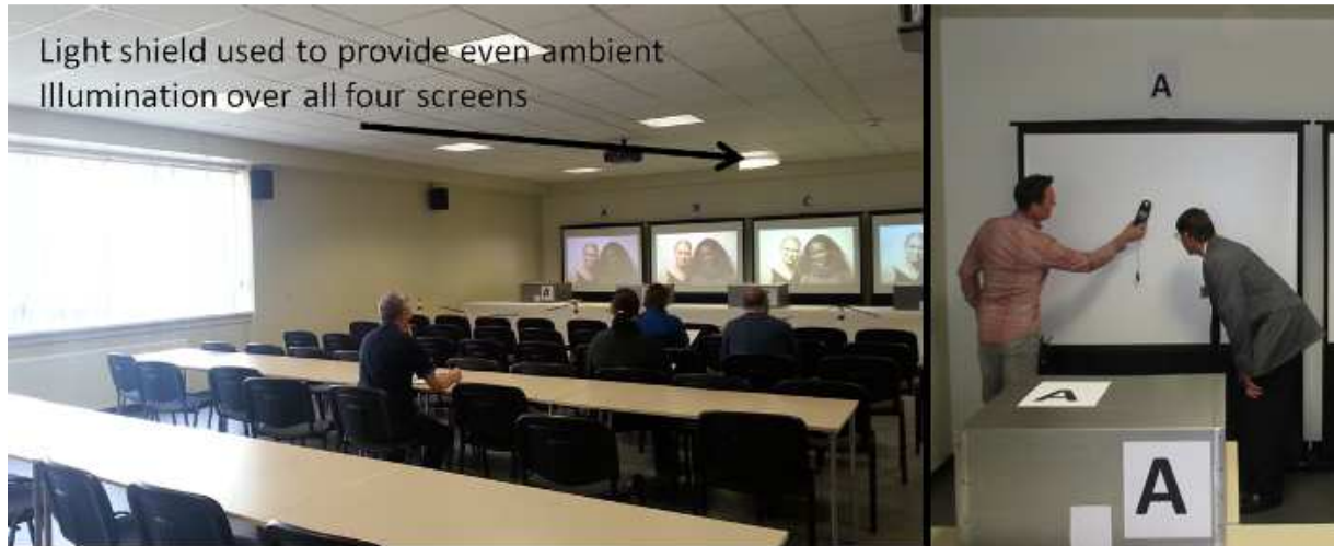
Figure 2: Room set up showing location of windows, projectors and light shield to provide uniform ambient illumination at the projector screens. Photo at right shows measurement of the ambient light levels.
