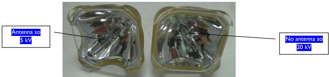
8) The replacement lamp has different **connection methods** over the original lamp used in the projector.
