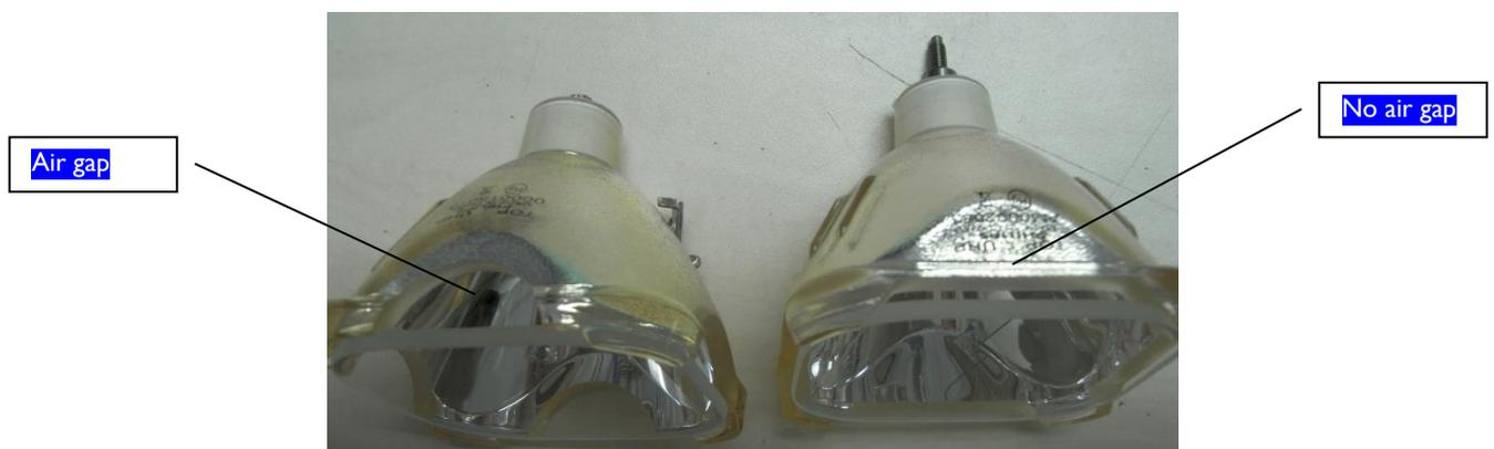
**6) The replacement lamps has non-identical **materials** and non-identical **coatings** over the original lamp used in the projector.**
