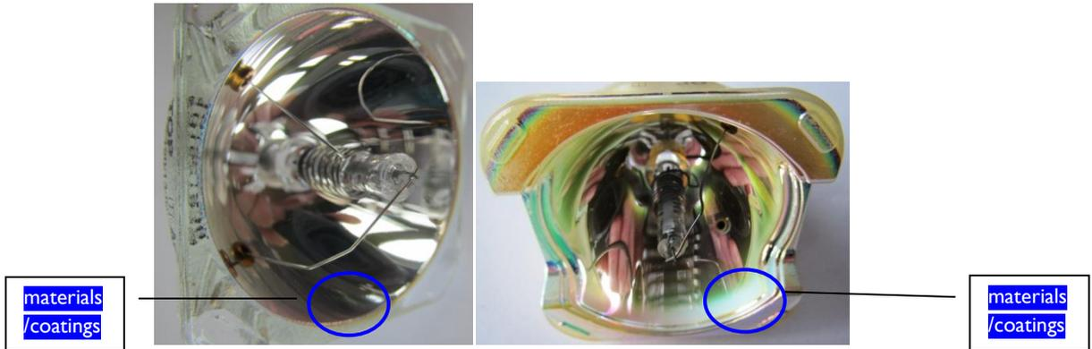
7) The replacement lamp has a different **ignition voltage** over the original lamp used in the projector. Lamps with metal “antenna” in the tube are 5 kV lamps. For some lamps, the antenna is in the front, for some lamps the antenna is in the rear.
