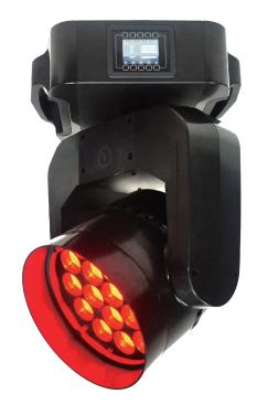
The SL WASH 350 LED Luminaire delivers an extremely bright homogenous beam with a large zoom range. The luminaire's 19 RGBW 15-watt LEDs deliver over 5,800 lumens of output and an extremely wide color palette. The large motorized zoom range of 8° to 40° provides designers with the freedom to use the SL WASH 350 as a special or as a wash luminaire.
