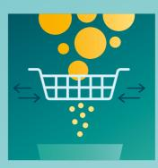
The fluorescent powder is removed in one of two ways. Using the dry technology method, the dust is sucked up using sieving or cyclones. In the wet technology method, the glass is washed and the powders are subsequently removed from the water.
