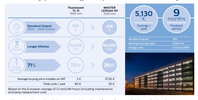
Choose Standard Output LEDtubes for a lower TCO with the best energy efficiency
