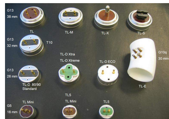
Fig. 4.8 Variety of different lamp caps employed with tubular fluorescent lamps.
