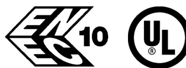
Fig. 15.58 ENEC and UL certification marks. The number in the ENEC mark indicates the country of the institute that has given the European approval.
