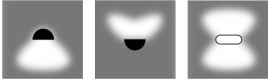
Fig. 15.35 From left to right: direct, indirect and direct-indirect types of luminaires.
