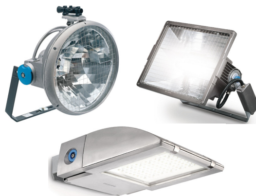
Fig. 15.57 Examples of floodlight light distributions. Top left: asymmetrical light distribution (floodlight with support for removable aiming telescope); top right: plane symmetrical light distribution about two planes; bottom: LED floodlight with asymmetrical light distribution.
