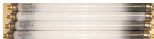
Fig. 4.5 Blackening of fluorescent tubes because of scattering of emitter material from the electrodes (no protecting ring).
