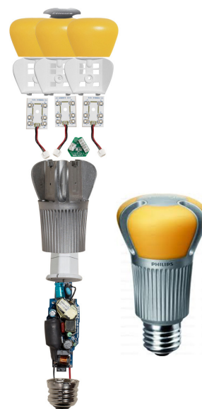
Fig. 11.15 Philips LED bulb producing high-quality white light with remote phosphor. Left: parts of the LED bulb, from bottom to top: lamp cap, electronic driver, heat sinks, two arrays with six LEDs, secondary optics, remote phosphor, top seal.
