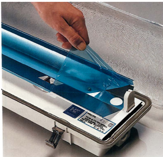
Fig. 15.27 Mirror reflector of sheet aluminium protected by a plastic film, which must be removed before use.
