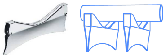
Fig. 15.15 Louvre design that provides omni-directional control of disturbing reflections in display screens.
