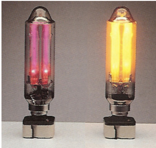
Fig. 7.3 Immediately after switch-on, a low-pressure sodium lamp emits just a little reddish light, which gradually changes to the familiar yellow sodium light when the lamp has fully warmed up.
