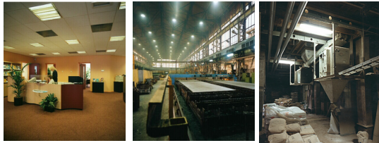
Fig. 15.30 Environments requiring (from left to right) luminaires with IP code 20, 54 and 65 respectively.
