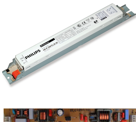
Fig. 13.12 Electronic ballast for fluorescent lamps. Below: the internal printed-circuit board.
