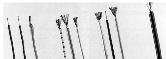
Fig. 15.32 Different types of electrical wiring used in luminaires. From left to right: solid core (3), stranded (3), stranded with heat-resistant insulation (3), and high-voltage ignition cable (1).
