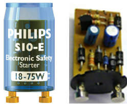
Fig. 13.3 Electronic starter as a direct replacement for the glow-switch starter.
