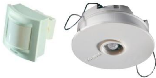
Fig. 16.4 Examples of occupancy detectors. Left: for wall mounting. Right: for recessed ceiling mounting (the small extendable cylinder around the motion sensor can be used to adjust the detection range).
