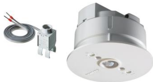
Fig. 16.3 Examples of photocells. Left: stand-alone cell for mounting on a tubular fluorescent lamp and wired directly to the dimming ballast. Right: Multimeter with photocell, occupancy detector (in the centre of the device) and IR receiver.
