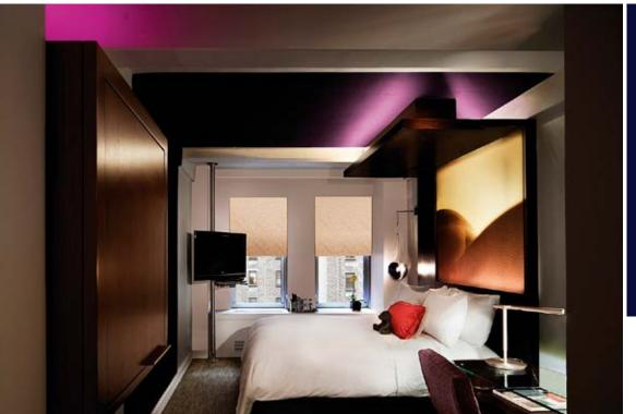
The LEDs illuminate banels which appear as art objects during the day and operate as light boxes at night.
