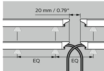
Mounting distance between modules for regular spacing of LED puck.
