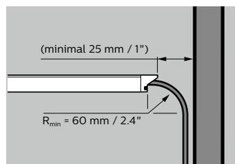
Mounting clearance from wall or rack with respect to minimum bending radius.
