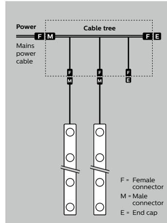
Module can be connected to power with either a power cable, a cable tree or a field installable connector\*. Any unused connector must be secured and sealed with an end cap. Otherwise the IP66 and UL rating for wet locations will be void. See Application Guide for detailed installation instructions.
