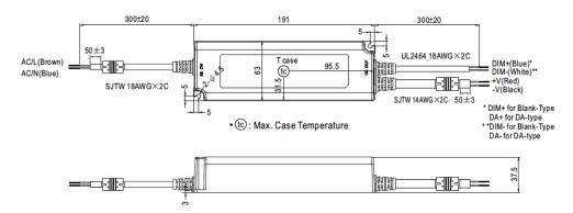
The power supply is IP67 certified in a plastic enclosure and can be mounted inside the chicken barn. Wires at the end are ~300mm long and need to be connected inside suitable junction boxes (standard catalog items).
