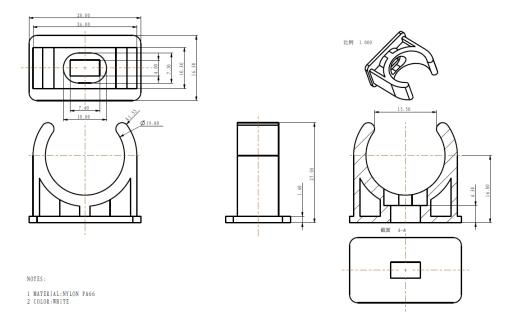
Number or clips needed for these standard clips and the way of mounting needs to be studied case by case. Orientation is not always fixed by these clips and should be solved in a different way (i.e. special bracket).
