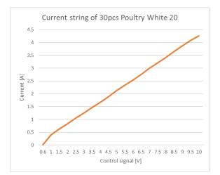
In the region of 1-10V the dimming behavior is linear, full off is achieved at a level of below ~0,6V.
