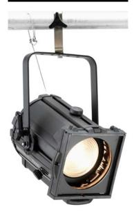
The Rama 150 Fresnel (1.0kW / 1.2kW, 150mm lens) provides an adjustable cone of light that has a soft edge, easily blended with adjacent beams to provide even illumination.
