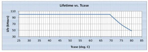
Failure rate info based upon field called rate data: < 0.2% per 1 KHr @  $\leq$  T case 80°C
