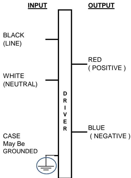
Input and output use lead-wires.
