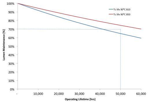
Lumen depreciation as a function of operating hours for I-life and Tc-life. 50,000 hours proven by certified laboratory.
