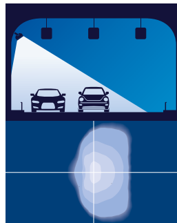
Typical 3 lane tunnel / cornice configuration
