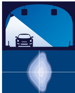
Typical 2 lane tunnel / cornice configuration
