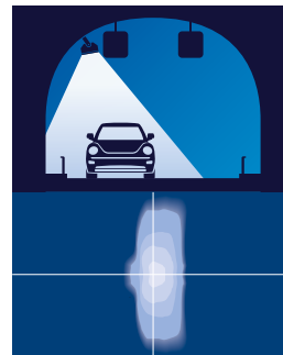
Typical 2 lane narrow tunnel / cornice configuration
