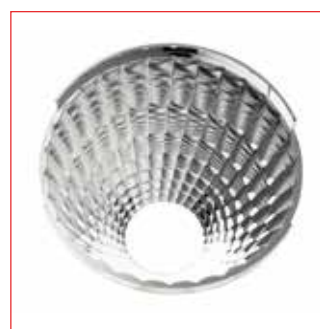
Flood Used for efficient highlighting of large objects or to emphasize a complete area. Beam angle: 34°-36°
