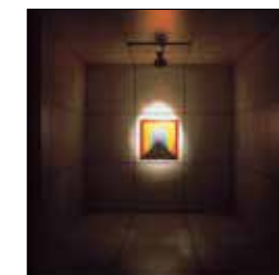
K2 is a spot which stands out due to its sharp transition to a minimal amount of spill light; this type of beam is excellent for creating theatrical and dramatic effects. This class is usually associated with very high-intensity beams.
