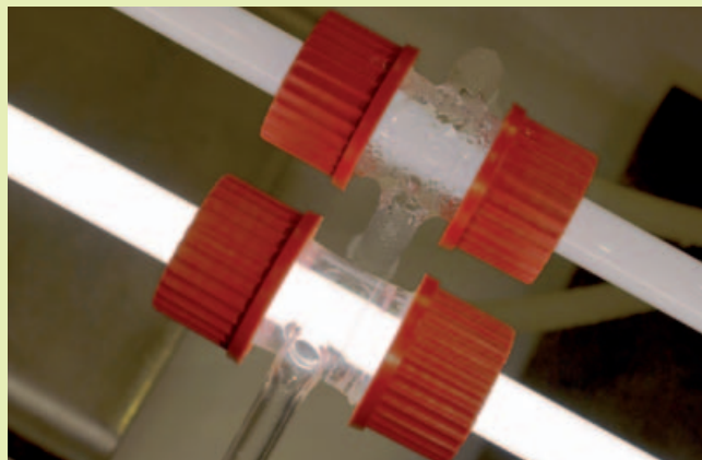
Figure 1: A cold spot is created on a fluorescent lamp by allowing cooling water to flow through a cell that is connected to a lamp. In the images, only the upper lamp is connected to the cooling water. In the left image, the mercury from the right side of the cooled lamp has sublimated on the cold spot (recognizable by the darker appearance), whereas in the right image also the mercury from the left side has sublimated on the cold spot. Apparently, the left side of the cooled lamp has the highest mercury concentration. Therefore it takes longer to sublimate all the mercury from the left side on the cold spot. The uncooled lamp stays equally bright along its entire length.
