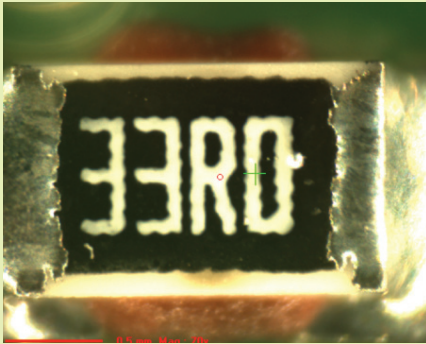
Fig. 1: the red circle shows a 30 µm measuring spot on the component of the PCB with the red rectangle in figure 2.
