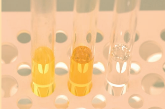
Fig. 2: Carius tubes filled with HCl + Fe(II) before (colourless) and after (yellow) reaction with Ce(IV). The orange colour represents a higher concentration of Ce(IV)-sulphate.
