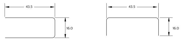
Mounting in cut-out in sheet matal (thickness 0.7 mm to 1.2 mm), tolerance +/-0.2 mm
