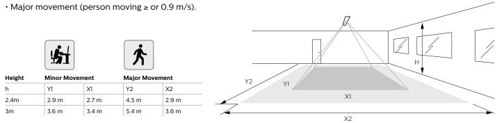
Note: Longer dimension of detection area (Y1, Y2) is parallel to longer dimension of EasyAir.
