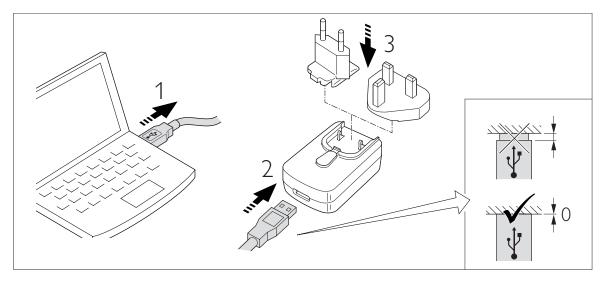
• Insert the power supply into the plug (the controller will automatically be enabled and operational).
