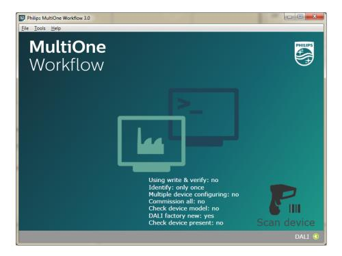
Scan the barcode on the device when you are in this screen. When the barcode was scanned successfully and the file is loaded, MultiOne Workflow continues with the configuration workflow.
