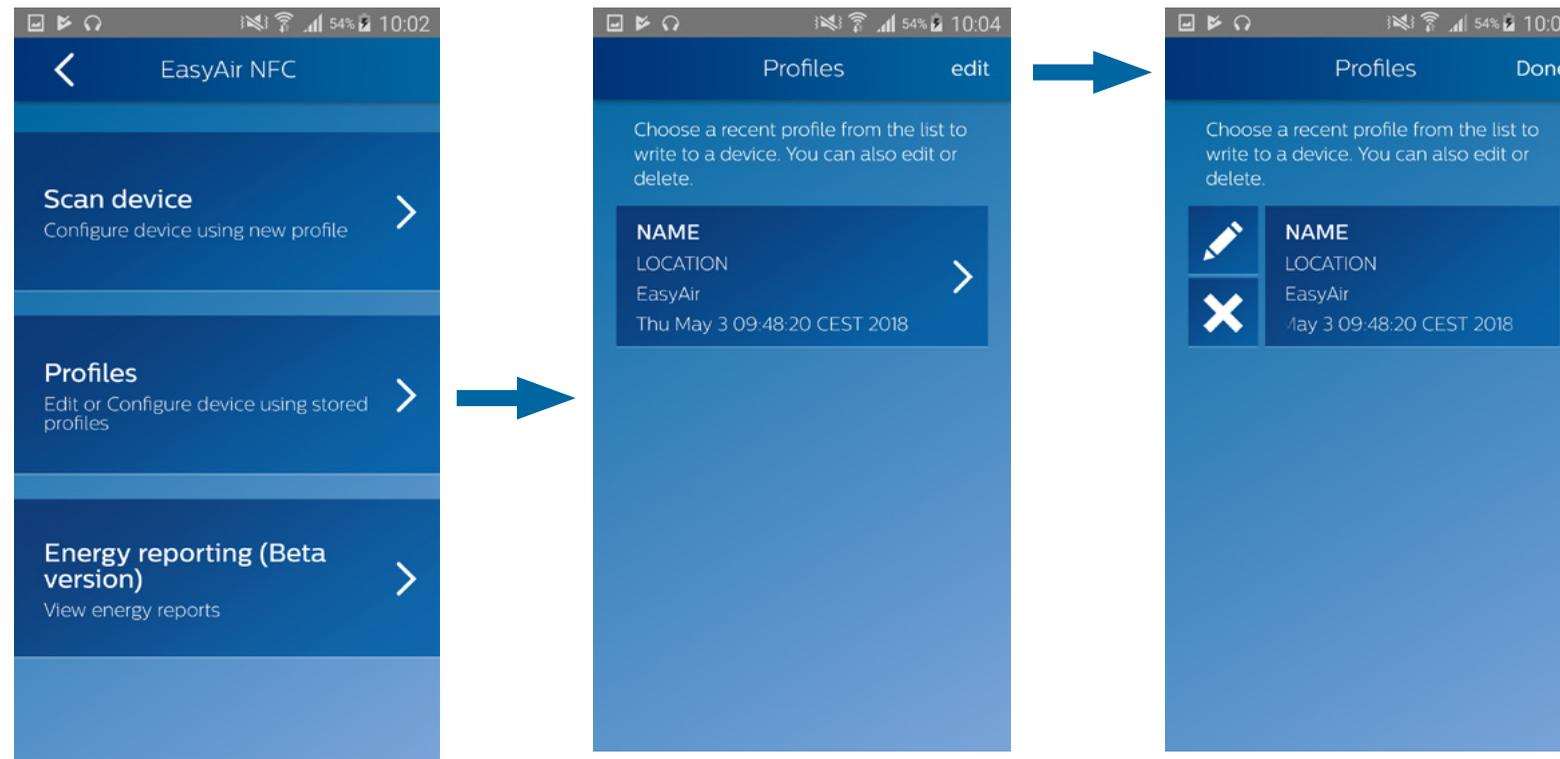
With the NFC App, the user can write back a profile to a single EasyAir sensor.
