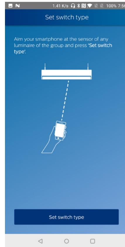
5. Aim the smartphone at any luminaire of the group and press **Set switch type**
