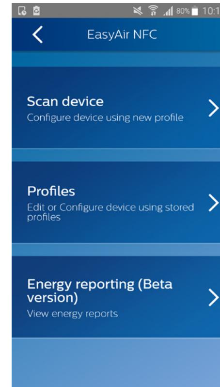
→ Access information about the device and configure the luminaire. This setup (profile) can be saved for re-use with other luminaires. Configure EasyAir by positioning phone near the NFC antenna of Android phone.
