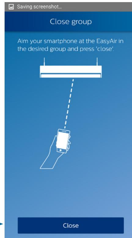
7. Aim the smartphone at the sensor of any luminaire of the group and press **Close**
