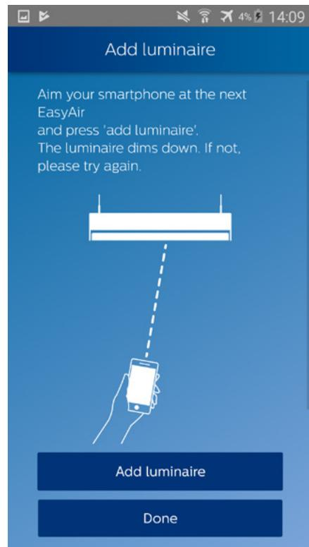
5. Aim the smartphone at the sensor of the luminaire to add in the group, and press **Add luminaire**. If the luminaire dims down, press **Done**.
