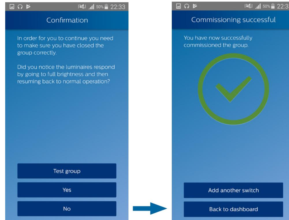
8. Check that the luminaires of the group went to full brightness before resuming to normal operation, indicating the group is closed
