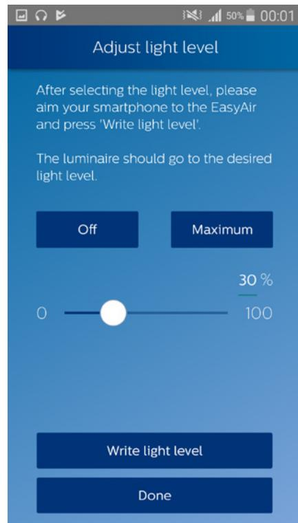
4. Set the desired light level: 30%. Once ready, aim the smartphone at the sensor of a luminaire of the group and press **Write light level**. Check that the luminaires went to the desired light level, then press **Done**.
