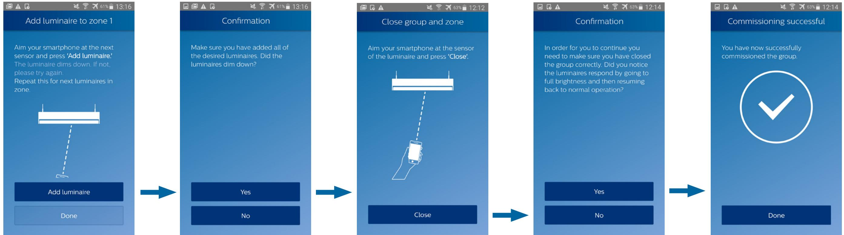
4. Aim the smartphone at luminaire 5, and press **Add luminaire**. If needed, repeat with other luminaires you want to add to Zone 1. Then, press **Done**.
