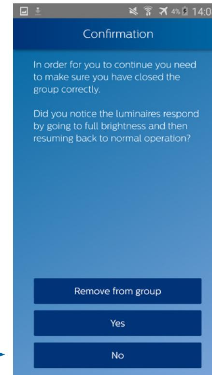
8. Check that all the luminaires of the group went to full brightness before going back to normal operation, indicating that the group is closed. Press **Yes**
