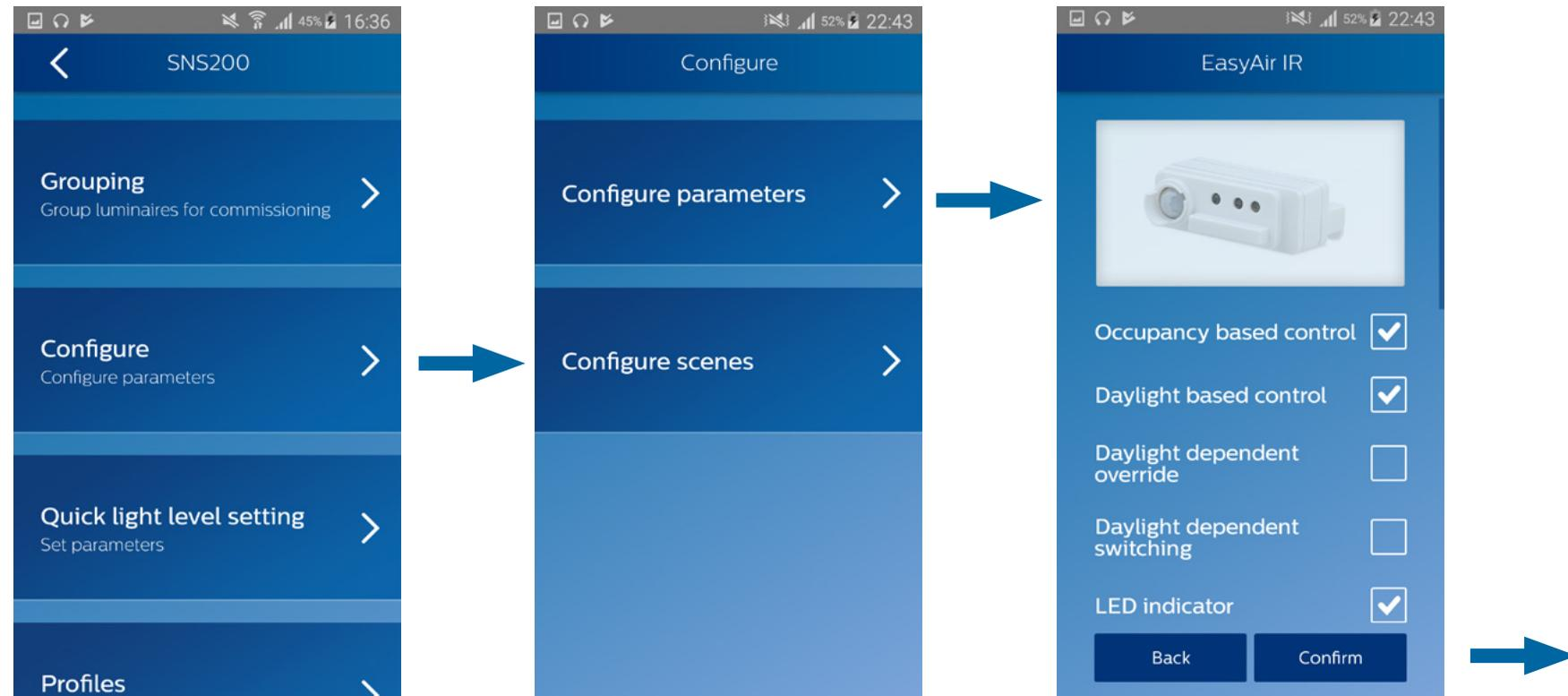
1. Open the *Configure parameters* submenu under *Configure* menu.
