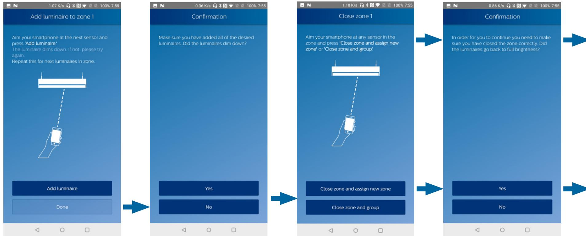
4. Aim smartphone at sensor 2 and **Add luminaire**. The luminaire will dim down implying it is added to zone 1. Then press **Done**.
