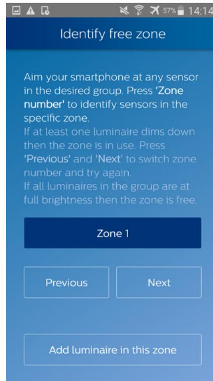
3. Select the zone the luminaire will be added to. In our case, the zones 1 and 2 are used already. Press **Next** to switch to Zone 3.
