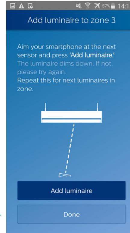
5. Aim the smartphone at luminaire 5, and press **Add luminaire**. If needed, repeat with other luminaires you want to add the new Zone 3. Then, press **Done**.
