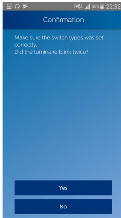
4. Check that the luminaires of the group blinked twice, indicating the switch type was set correctly
