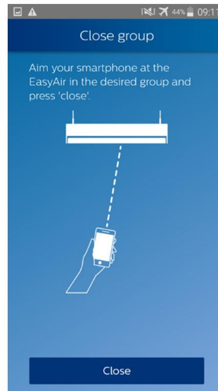
7. Aim the smartphone to the sensor of any luminaire of the group and press **Close**
