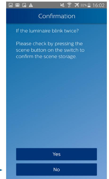
8. Check if the luminaires of the group blinked twice, and that the scene is properly stored on the sensor and is associated to the switch.
