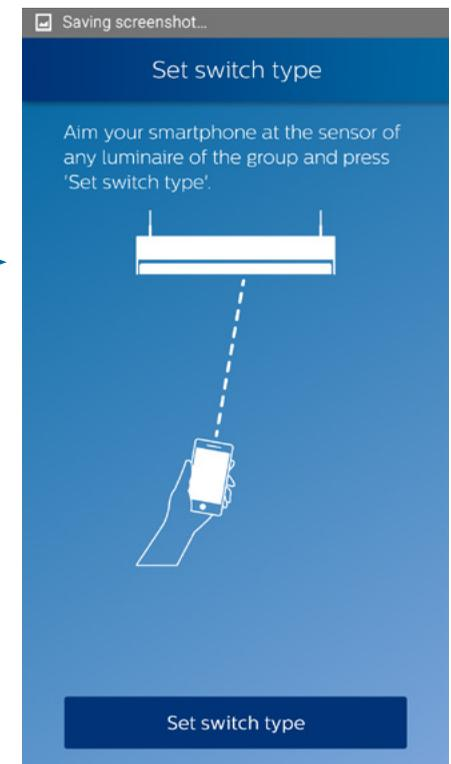
3. Aim your smartphone to the sensor of any luminaire of the group, and press **Set switch type**
