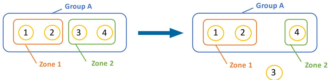
Note: to change a luminaire's zone, the user will first have to remove it from a group, then add it to the desired zone – please refer “Add luminaire to a zone” in EasyAir Industry IR app.
