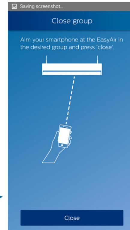
7. Aim your smartphone at the sensor of any luminaire of the group and press **Close**
