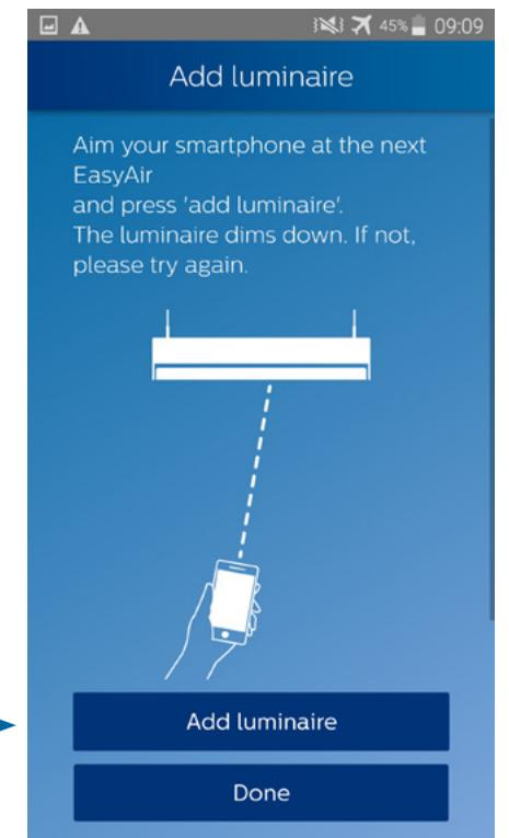
4. Aim the smartphone at the sensor of luminaire 2, and press **Add luminaire**.
