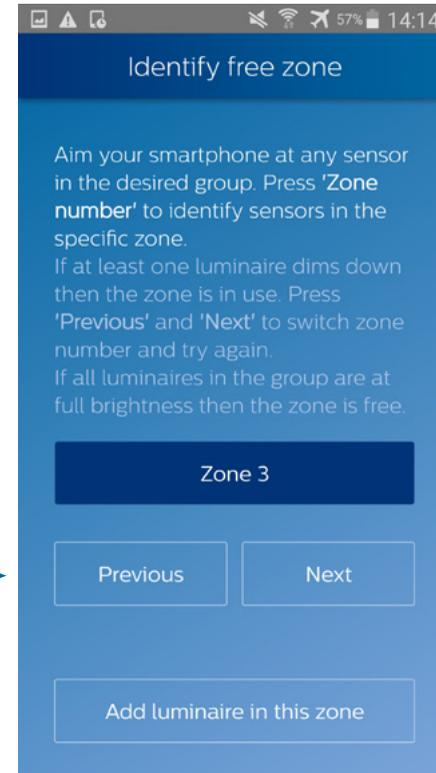
4. Check that none of the luminaires dim down (meaning that zone 3 is indeed free), and press **Add luminaire in this zone**.
