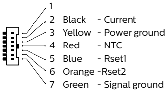
JST connector (driver side) pin layout
