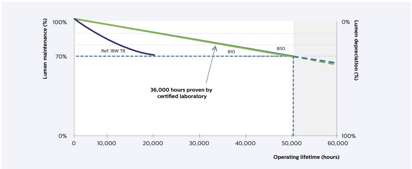
Lumen depreciation as a function of operating hours for LED Strip 1 ft 650 lm LV3.
