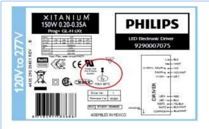
Figure 18 - Product label indicating Tc point H-can driver
