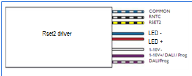
Figure 3 – Rset2 driver lead wire color code definition
