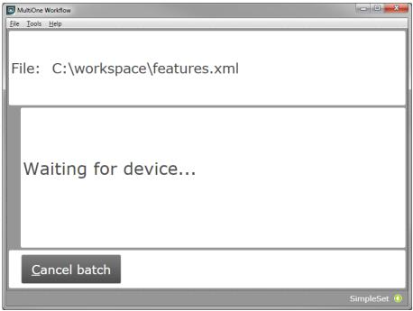
Use **Cancel batch** to go to the main application window. To continue hold the SimpleSet® interface close to the device.
