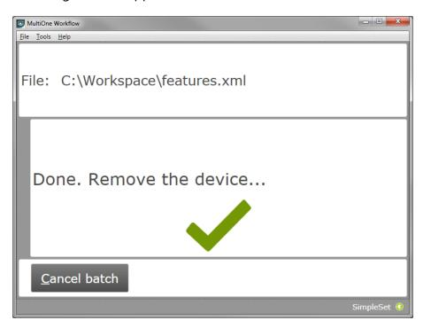
Move the SimpleSet<sup>®</sup> interface away from the device, MultiOne will then show the waiting for device view as explained in **5.5.2**
