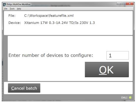
If in the preferences the configuration mode was set to **Batch size**, MultiOne Workflow will display a window in which the number of devices for this batch can be entered. The minimum number of devices is 1.
