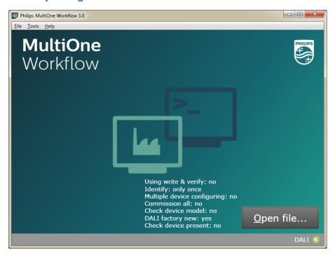
Feature file and schedule file are both Workflow files. If the **DALI protocol** is used and the configuration mode is **Single shot**, then Workflow accepts both type of Workflow files. Otherwise, Workflow will only accept feature files. To open a file, select **File > Open...** or click **Open file...** . Select a file and click **Open**.
