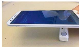
Click 'Program EasySense' and place the back of the smartphone onto the sensor NFC antenna again to enable NFC communication. NFC communication might take a few seconds, do not move until the next screen shows.
