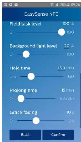
After hearing a beep, the following screen will appear. Key parameters can be configured using the sliding bar or by typing in the exact number on the right. After configuration, press "Confirm."
