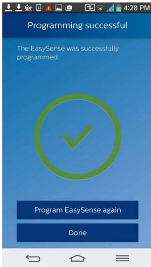
After programming successfully, a green check mark will appear on the screen. More sensors can be programmed with the same setting by pressing “Program EasySense again”. Or press “Done” to finish configuration.
