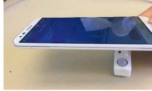
Place the back of the smartphone (where the NFC reader locates) onto the sensor NFC antenna (almost touching) to enable NFC communication. NFC communication might take a few seconds, do not move until the next screen appears.
