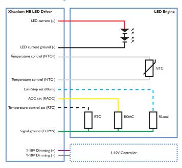
Note: do not connect Signal ground and LED current ground on LED engine
