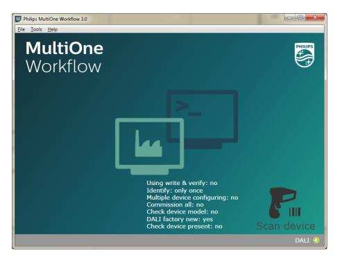
Scan the barcode on the device when you are in this screen. When the barcode was scanned successfully and the file is loaded, MultiOne Workflow continues with the configuration workflow.
