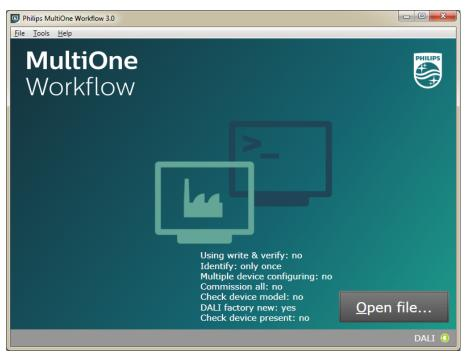
Feature file and schedule file are both Workflow files. If the **DALI protocol** is used and the configuration mode is **Single shot**, then Workflow accepts both type of Workflow files. Otherwise, Workflow will only accept feature files. To open a file, select **File**  $\rightarrow$  **Open...** or click **Open file...** . Select a file and click **Open**.
